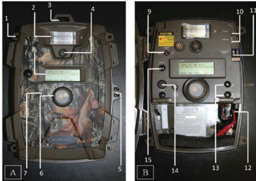
Figure 1. Diagram of the external (A) and internal (B) components of a Moultrie Game Spy trail camera. 1. Mounting Cord Lug 2. Electronic Flash 3. Viewfinder 4. Camera Lens 5. Lockable Latch 6. Infrared Sensor 7. Status Light 8. LCD Status Display 9. Power On/Off Button 10. TV and USB Ports 11. SD Memory Card Slot 12. Battery Compartment 13. Change Buttons 14. Mode Button 15. Select Button.
