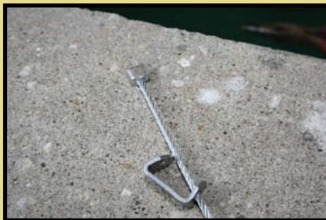
Figure 3. Single ferrule crimped to end of snare cable.
