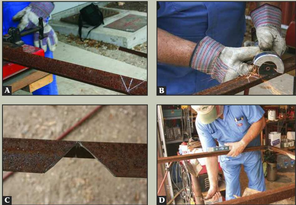
A piece of angle iron marked for cutting (A). After cutting (B and C), the iron can be heated and bent to form the desired configuration (D). The bracket is then welded. Designs may differ, depending on the door style.
